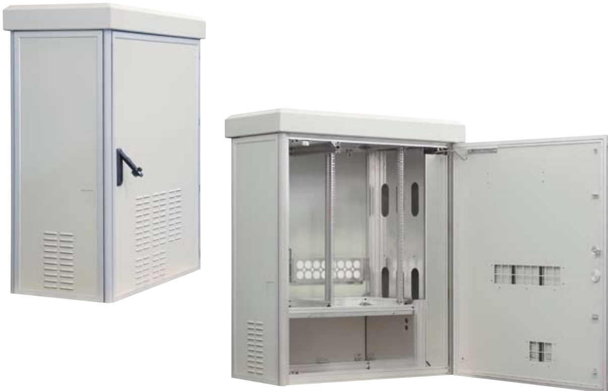
Cabinet based on standard SZD type; aluminium doors and shields panels were replaced by aluminium sheet.
