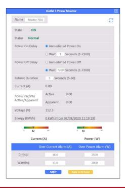
Take Outlet4 for example (Set Power ON/OFF Delay=3 seconds /Reboot Duration=10 seconds), when you select Action "Off Delay" and click Apply. Outlet4 will power off after 3 seconds.
