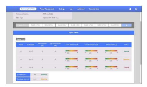
The main page shows a graphic representation of the Power Strip outlets and inputs status as described below:
