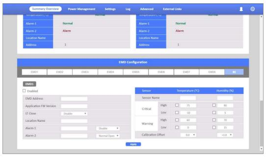
SCHNEIKEL PDU supports 8 EMD sensors in cascade each one with 2 digital inputs to set 2 alarms for each EMD 31 sensor. There are 3 options(Normal Open/Normal Close/Disable) of the EMD sensor. If you set "Normal Open", the EMD sensor will become "Warning" (Yellow light) when closed.
