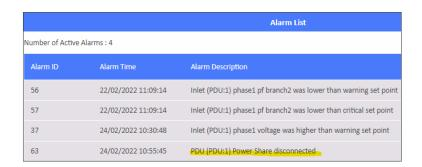
**Step 12:** The related log and trap will be recorded on the Log of Event Log webpage and NMS. The log and trap will be "Warning: Inlet (PDU:1) Active/Main Power change to Inactive".
