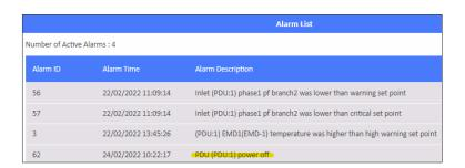
**Step 7:** The related log and trap will be recorded on the **Log** of **Event Log** webpage and NMS. The log and trap will be "warning: Inlet (PDU:1) Acv e/Main Power change to Acv e/Backup Power".
