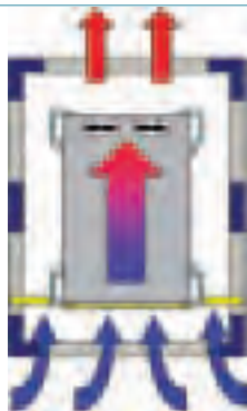
Hot And Cold Air Segregation
